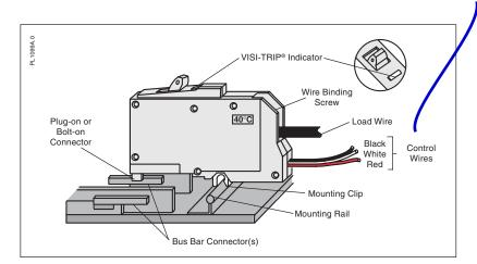
4. Except for remotely operated connections, QO(B)-PL remotely operated circuit breakers are installed in a panelboard/load center the same as conventional QO(B) circuit breakers.
