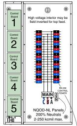
Square D NQOD-NL MB Panel with LvnTec sidecar. Standard SCP Main Breaker: 225 Amp. - 65k AIR - M225 Square D# MJGP36225
