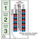
Main Lug Only)-MLO option Remove Back fed main and top feed as a MLO to gain 3 circuits. Feed from a protected disconnect.
